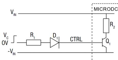
$D_1$  (eg 1N4001) is required to provide high impedance when the signal is low. From the WRA-YLS-3W specification, the drive current to operate this function is recommended to be 6mA, and hence the value of  $R_1$  can be derived as follows:
